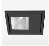
Recessed luminaire with LED, rated life of the LED L80/B10 > 50000 h, chromaticity tolerance 2 SDCM (initial), reflector with asymmetrical light distribution pattern, reflector pure aluminium 99,99% in MIRO-Silver®, swivel angle 30°, luminaire housing sheet steel, powder-coated, stratoblack, separate driver unit
