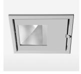
Recessed luminaire with LED, rated life of the LED L80/B10 > 50000 h, colour rendering index CRI > 96, chromaticity tolerance 2 SDCM (initial), reflector with asymmetrical light distribution pattern, reflector pure aluminium 99,99% in MIRO-Silver®, swivel angle 30°, luminaire housing sheet steel, powder-coated, stratosilver, separate driver unit
