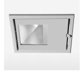
Recessed luminaire with LED, rated life of the LED L80/B10 > 50000 h, chromaticity tolerance 2 SDCM (initial), reflector with asymmetrical light distribution pattern, reflector pure aluminium 99,99% in MIRO-Silver®, swivel angle 30°, luminaire housing sheet steel, powder-coated, stratosilver, separate driver unit
