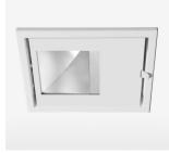
Recessed luminaire with LED, rated life of the LED L80/B10 > 50000 h, colour rendering index CRI > 96, chromaticity tolerance 2 SDCM (initial), reflector with asymmetrical light distribution pattern, reflector pure aluminium 99,99% in MIRO-Silver®, swivel angle 30°, luminaire housing sheet steel, powder-coated, stratowhite, separate driver unit
