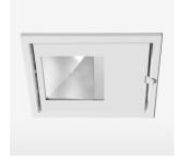
Recessed luminaire with LED, rated life of the LED L80/B10 > 50000 h, colour rendering index CRI > 96, chromaticity tolerance 2 SDCM (initial), reflector with asymmetrical light distribution pattern, reflector pure aluminium 99,99% in MIRO-Silver®, swivel angle 30°, luminaire housing sheet steel, powder-coated, stratowhite, separate driver unit
