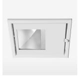
Recessed luminaire with LED, rated life of the LED L80/B10 > 50000 h, colour rendering index CRI > 96, chromaticity tolerance 3 SDCM (initial), reflector with asymmetrical light distribution pattern, reflector pure aluminium 99,99% in MIRO-Silver®, swivel angle 30°, luminaire housing sheet steel, powdercoated, stratowhite, separate driver unit
