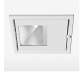
Recessed luminaire with LED, rated life of the LED L80/B10 > 50000 h, colour rendering index CRI > 96, chromaticity tolerance 3 SDCM (initial), reflector with asymmetrical light distribution pattern, reflector pure aluminium 99,99% in MIRO-Silver®, swivel angle 30°, luminaire housing sheet steel, powder-coated, stratowhite, separate driver unit
