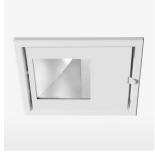
Recessed luminaire with LED, rated life of the LED L80/B10 > 50000 h, chromaticity tolerance 2 SDCM (initial), reflector with asymmetrical light distribution pattern, reflector pure aluminium 99,99% in MIRO-Silver®, swivel angle 30°, luminaire housing sheet steel, powder-coated, stratowhite, separate driver unit
