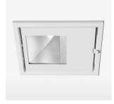
Recessed luminaire with LED, rated life of the LED L80/B10 > 50000 h, chromaticity tolerance 2 SDCM (initial), reflector with asymmetrical light distribution pattern, reflector pure aluminium 99,99% in MIRO-Silver®, swivel angle 30°, luminaire housing sheet steel, powder-coated, stratowhite, separate driver unit
