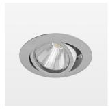
Recessed luminaire with LED, rated life of the LED L80/B10 > 50000 h, colour rendering index CRI > 96, chromaticity tolerance 2 SDCM (initial), rotation-symmetrical reflector with circular light distribution pattern, reflector pure aluminium 99,99% in MIRO-Silver®, segmented and faceted, 3D lens silicon to reduce the proportion of scattered light, die-cast aluminium, powder-coated, rotation angle , swivel angle +25° / -25°, stratosilver,
