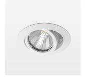
Recessed luminaire with LED, rated life of the LED L80/B10 > 50000 h, colour rendering index CRI > 80, chromaticity tolerance 3 SDCM (initial), rotation-symmetrical reflector with circular light distribution pattern, reflector pure aluminium 99,99% in MIRO-Silver®, segmented and faceted, 3D lens silicon to reduce the proportion of scattered light, die-cast aluminium, powder-coated, rotation angle , swivel angle +25° / -25°, stratowhite,
