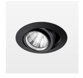
Recessed luminaire with LED, rated life of the LED L80/B10 > 50000 h, colour rendering index CRI > 90, chromaticity tolerance 2 SDCM (initial), rotation-symmetrical reflector with circular light distribution pattern, reflector pure aluminium 99,99% in MIRO-Silver®, segmented and faceted, 3D lens silicon to reduce the proportion of scattered light, die-cast aluminium, powder-coated, rotation angle , swivel angle +25° / -25°, stratoblack,
