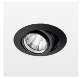
Recessed luminaire with LED, rated life of the LED L80/B10 > 50000 h, colour rendering index CRI > 90, chromaticity tolerance 2 SDCM (initial), rotation-symmetrical reflector with circular light distribution pattern, reflector pure aluminium 99,99% in MIRO-Silver®, segmented and faceted, 3D lens silicon to reduce the proportion of scattered light, die-cast aluminium, powder-coated, rotation angle, swivel angle +25° / -25°, stratoblack,
