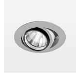
Recessed luminaire with LED, rated life of the LED L80/B10 > 50000 h, colour rendering index CRI > 80, chromaticity tolerance 2 SDCM (initial), rotation-symmetrical reflector with circular light distribution pattern, reflector pure aluminium 99,99% in MIRO-Silver®, segmented and faceted, 3D lens silicon to reduce the proportion of scattered light, die-cast aluminium, powder-coated, rotation angle , swivel angle  $\pm 25^{\circ}$  /  $\pm 25^{\circ}$ , stratosilver,
