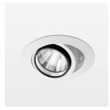
Recessed luminaire with LED, rated life of the LED L80/B10 > 50000 h, colour rendering index CRI > 80, chromaticity tolerance 2 SDCM (initial), rotation-symmetrical reflector with circular light distribution pattern, reflector pure aluminium 99,99% in MIRO-Silver®, segmented and faceted, 3D lens silicon to reduce the proportion of scattered light, die-cast aluminium, powder-coated, rotation angle , swivel angle +25°/ -25°, stratowhite,
