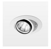
Recessed luminaire with LED, rated life of the LED L80/B10 > 50000 h, colour rendering index CRI > 80, chromaticity tolerance 2 SDCM (initial), rotation-symmetrical reflector with circular light distribution pattern, reflector pure aluminium 99,99% in MIRO-Silver®, segmented and faceted, 3D lens silicon to reduce the proportion of scattered light, die-cast aluminium, powder-coated, rotation angle , swivel angle  $+25^{\circ}/-25^{\circ}$ , stratowhite,
