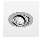
Recessed luminaire with LED, rated life of the LED L80/B10 > 50000 h, colour rendering index CRI > 90, chromaticity tolerance 2 SDCM (initial), rotation-symmetrical reflector with circular light distribution pattern, reflector pure aluminium 99,99% in MIRO-Silver®, segmented and faceted, 3D lens silicon to reduce the proportion of scattered light, die-cast aluminium, powder-coated, rotation angle , swivel angle  $\pm 25^{\circ}/ -25^{\circ}$ , stratosilver,
