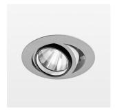
Recessed luminaire with LED, rated life of the LED L80/B10 > 50000 h, colour rendering index CRI > 80, chromaticity tolerance 2 SDCM (initial), rotation-symmetrical reflector with circular light distribution pattern, reflector pure aluminium 99,99% in MIRO-Silver®, segmented and faceted, 3D lens silicon to reduce the proportion of scattered light, die-cast aluminium, powder-coated, rotation angle, swivel angle +25°/-25°, stratosilver,
