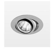
Recessed luminaire with LED, rated life of the LED L80/B10 > 50000 h, colour rendering index CRI > 80, chromaticity tolerance 2 SDCM (initial), rotationsymmetrical reflector with circular light distribution pattern, reflector pure aluminium 99,99% in MIRO-Silver®, segmented and faceted, 3D lens silicon to reduce the proportion of scattered light, die-cast aluminium, powder-coated, rotation angle , swivel angle +25°/ -25°, stratosilver,
