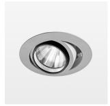
Recessed luminaire with LED, rated life of the LED L80/B10 > 50000 h, colour rendering index CRI > 96, chromaticity tolerance 2 SDCM (initial), rotation-symmetrical reflector with circular light distribution pattern, reflector pure aluminium 99,99% in MIRO-Silver®, segmented and faceted, 3D lens silicon to reduce the proportion of scattered light, die-cast aluminium, powder-coated, rotation angle, swivel angle +25°/-25°, stratosilver,
