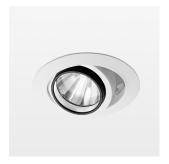
Recessed luminaire with LED, rated life of the LED L80/B10 > 50000 h, colour rendering index CRI > 90, chromaticity tolerance 2 SDCM (initial), rotation-symmetrical reflector with circular light distribution pattern, reflector pure aluminium 99,99% in MIRO-Silver®, segmented and faceted, 3D lens silicon to reduce the proportion of scattered light, die-cast aluminium, powder-coated, rotation angle , swivel angle  $\pm 25^{\circ}/ -25^{\circ}$ , stratowhite,
