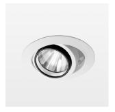
Recessed luminaire with LED, rated life of the LED L80/B10 > 50000 h, colour rendering index CRI > 90, chromaticity tolerance 2 SDCM (initial), rotation-symmetrical reflector with circular light distribution pattern, reflector pure aluminium 99,99% in MIRO-Silver®, segmented and faceted, 3D lens silicon to reduce the proportion of scattered light, die-cast aluminium, powder-coated, rotation angle , swivel angle  $+25^{\circ}/-25^{\circ}$ , stratowhite,
