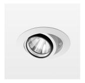
Recessed luminaire with LED, rated life of the LED L80/B10 > 50000 h, colour rendering index CRI > 96, chromaticity tolerance 2 SDCM (initial), rotation-symmetrical reflector with circular light distribution pattern, reflector pure aluminium 99,99% in MIRO-Silver®, segmented and faceted, 3D lens silicon to reduce the proportion of scattered light, die-cast aluminium, powder-coated, rotation angle , swivel angle  $+25^{\circ}/-25^{\circ}$ , stratowhite,
