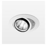
Recessed luminaire with LED, rated life of the LED L80/B10 > 50000 h, colour rendering index CRI > 96, chromaticity tolerance 2 SDCM (initial), rotation-symmetrical reflector with circular light distribution pattern, reflector pure aluminium 99,99% in MIRO-Silver®, segmented and faceted, 3D lens silicon to reduce the proportion of scattered light, die-cast aluminium, powder-coated, rotation angle, swivel angle +25°/-25°, stratowhite,
