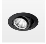
Recessed luminaire with LED, rated life of the LED L80/B10 > 50000 h, colour rendering index CRI > 80, chromaticity tolerance 2 SDCM (initial), rotation-symmetrical reflector with circular light distribution pattern, reflector pure aluminium 99,99% in MIRO-Silver®, segmented and faceted, 3D lens silicon to reduce the proportion of scattered light, die-cast aluminium, powder-coated, rotation angle, swivel angle +25°/-25°, stratoblack,
