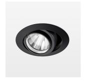
Recessed luminaire with LED, rated life of the LED L80/B10 > 50000 h, colour rendering index CRI > 80, chromaticity tolerance 2 SDCM (initial), rotation-symmetrical reflector with circular light distribution pattern, reflector pure aluminium 99,99% in MIRO-Silver®, segmented and faceted, 3D lens silicon to reduce the proportion of scattered light, die-cast aluminium, powder-coated, rotation angle , swivel angle  $+25^{\circ}/-25^{\circ}$ , stratoblack,
