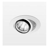
Recessed luminaire with LED, rated life of the LED L80/B10 > 50000 h, colour rendering index CRI > 90, chromaticity tolerance 2 SDCM (initial), rotation-symmetrical reflector with circular light distribution pattern, reflector pure aluminium 99,99% in MIRO-Silver®, segmented and faceted, 3D lens silicon to reduce the proportion of scattered light, die-cast aluminium, powder-coated, rotation angle , swivel angle  $+25^{\circ}/-25^{\circ}$ , stratowhite,
