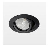
Recessed luminaire with LED, rated life of the LED L80/B10 > 50000 h, colour rendering index CRI > 80, chromaticity tolerance 2 SDCM (initial), reflector with circular light distribution pattern, reflector pure aluminium 99,99% in MIRO-Silver®, segmented and faceted, 3D lens silicon to reduce the proportion of scattered light, die-cast aluminium, powder-coated, rotation angle , swivel angle  $\pm 25^{\circ}$  /  $\pm 25^{\circ}$ , stratoblack,
