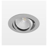
Recessed luminaire with LED, rated life of the LED L80/B10 > 50000 h, colour rendering index CRI > 90, chromaticity tolerance 2 SDCM (initial), reflector with circular light distribution pattern, reflector pure aluminium 99,99% in MIRO-Silver®, segmented and faceted, 3D lens silicon to reduce the proportion of scattered light, die-cast aluminium, powder-coated, rotation angle , swivel angle  $\pm 25^{\circ}$  /  $\pm 25^{\circ}$ , stratosilver,
