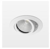
Recessed luminaire with LED, rated life of the LED L80/B10 > 50000 h, colour rendering index CRI > 80, chromaticity tolerance 2 SDCM (initial), reflector with circular light distribution pattern, reflector pure aluminium 99,99% in MIRO-Silver®, segmented and faceted, 3D lens silicon to reduce the proportion of scattered light, die-cast aluminium, powder-coated, rotation angle , swivel angle  $\pm 25^{\circ}$  /  $\pm 25^{\circ}$ , stratowhite,
