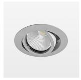
Recessed luminaire with LED, rated life of the LED L80/B10 > 50000 h, colour rendering index CRI > 90, chromaticity tolerance 2 SDCM (initial), reflector with circular light distribution pattern, reflector pure aluminium 99,99% in MIRO-Silver®, segmented and faceted, 3D lens silicon to reduce the proportion of scattered light, die-cast aluminium, powder-coated, rotation angle , swivel angle  $\pm 25^{\circ}$  /  $\pm 25^{\circ}$ , stratosilver,
