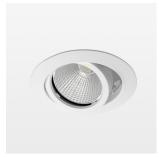
Recessed luminaire with LED, rated life of the LED L80/B10 > 50000 h, colour rendering index CRI > 96, chromaticity tolerance 2 SDCM (initial), reflector with circular light distribution pattern, reflector pure aluminium 99,99% in MIRO-Silver®, segmented and faceted, 3D lens silicon to reduce the proportion of scattered light, die-cast aluminium, powder-coated, rotation angle , swivel angle +25° / -25°, stratowhite,
