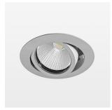
Recessed luminaire with LED, rated life of the LED L80/B10 > 50000 h, colour rendering index CRI > 80, chromaticity tolerance 2 SDCM (initial), reflector with circular light distribution pattern, reflector pure aluminium 99,99% in MIRO-Silver®, segmented and faceted, 3D lens silicon to reduce the proportion of scattered light, die-cast aluminium, powder-coated, rotation angle , swivel angle  $\pm 25^{\circ}$  /  $\pm 25^{\circ}$ , stratosilver,
