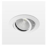
Recessed luminaire with LED, rated life of the LED L80/B10 > 50000 h, colour rendering index CRI > 80, chromaticity tolerance 2 SDCM (initial), reflector with circular light distribution pattern, reflector pure aluminium 99,99% in MIRO-Silver®, segmented and faceted, die-cast aluminium, powder-coated, rotation angle , swivel angle +25° / -25°, stratowhite,
