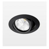
Recessed luminaire with LED, rated life of the LED L80/B10 > 50000 h, colour rendering index CRI > 96, chromaticity tolerance 2 SDCM (initial), reflector with oval light distribution pattern, reflector pure aluminium 99,99% in MIRO-Silver®, segmented, die-cast aluminium, powder-coated, rotation angle , swivel angle +25° / -25°, stratoblack,
