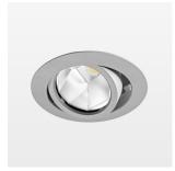
Recessed luminaire with LED, rated life of the LED L80/B10 > 50000 h, colour rendering index CRI > 96, chromaticity tolerance 2 SDCM (initial), reflector with oval light distribution pattern, reflector pure aluminium 99,99% in MIRO-Silver®, segmented, die-cast aluminium, powder-coated, rotation angle , swivel angle  $\pm 25^{\circ}$  /  $\pm 25^{\circ}$ , stratosilver,
