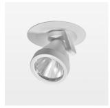
Semi-recessed luminaire with LED, rated life of the LED L80/B10 > 50000 h, colour rendering index CRI > 96, chromaticity tolerance 2 SDCM (initial), rotation-symmetrical reflector with circular light distribution pattern, reflector pure aluminium 99,99% in MIRO-Silver®, segmented and faceted, 3D lens silicon to reduce the proportion of scattered light, die-cast aluminium, powder-coated, rotation angle 400°, swivel angle +85° / -85°, stratowhite, separate driver unit
