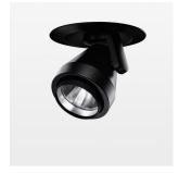
Semi-recessed luminaire with LED, rated life of the LED L80/B10 > 50000 h, colour rendering index CRI > 80, chromaticity tolerance 2 SDCM (initial), rotation-symmetrical reflector with circular light distribution pattern, reflector pure aluminium 99,99% in MIRO-Silver®, segmented and faceted, 3D lens silicon to reduce the proportion of scattered light, die-cast aluminium, powdercoated, rotation angle 400°, swivel angle +85° / -85°, stratoblack, separate driver unit
