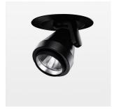
Semi-recessed luminaire with LED, rated life of the LED L80/B10 > 50000 h, colour rendering index CRI > 96, chromaticity tolerance 2 SDCM (initial), rotation-symmetrical reflector with circular light distribution pattern, reflector pure aluminium 99,99% in MIRO-Silver®, segmented and faceted, 3D lens silicon to reduce the proportion of scattered light, die-cast aluminium, powdercoated, rotation angle 400°, swivel angle +85° / -85°, stratoblack, separate driver unit
