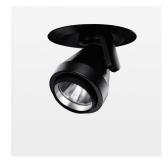
Semi-recessed luminaire with LED, rated life of the LED L80/B10 > 50000 h, colour rendering index CRI > 96, chromaticity tolerance 2 SDCM (initial), rotation-symmetrical reflector with circular light distribution pattern, reflector pure aluminium 99,99% in MIRO-Silver®, segmented and faceted, 3D lens silicon to reduce the proportion of scattered light, die-cast aluminium, powdercoated, rotation angle 400°, swivel angle +85° / -85°, stratoblack, separate driver unit
