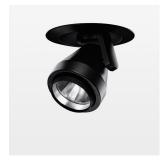
Semi-recessed luminaire with LED, rated life of the LED L80/B10 > 50000 h, colour rendering index CRI > 90, chromaticity tolerance 2 SDCM (initial), rotation-symmetrical reflector with circular light distribution pattern, reflector pure aluminium 99,99% in MIRO-Silver®, segmented and faceted, 3D lens silicon to reduce the proportion of scattered light, die-cast aluminium, powdercoated, rotation angle 400°, swivel angle +85° / -85°, stratoblack, separate driver unit
