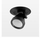
Semi-recessed luminaire with LED, rated life of the LED L80/B10 > 50000 h, colour rendering index CRI > 90, chromaticity tolerance 2 SDCM (initial), reflector with circular light distribution pattern, reflector pure aluminium 99,99% in MIRO-Silver®, segmented and faceted, 3D lens silicon to reduce the proportion of scattered light, die-cast aluminium, powder-coated, rotation angle 400°, swivel angle +85° / -85°, stratoblack, separate driver unit
