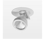
Semi-recessed luminaire with LED, rated life of the LED L80/B10 > 50000 h, colour rendering index CRI > 96, chromaticity tolerance 2 SDCM (initial), reflector with circular light distribution pattern, reflector pure aluminium 99,99% in MIRO-Silver®, segmented and faceted, 3D lens silicon to reduce the proportion of scattered light, die-cast aluminium, powder-coated, rotation angle 400°, swivel angle +85°/-85°, stratowhite, potentiometer to adjust the brightness, separate driver unit
