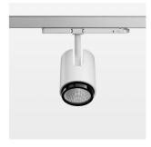
Surface-mounted luminaire with LED, rated life of the LED L80/B10 > 50000 h, chromaticity tolerance 3 SDCM (initial), , reflector with circular light distribution pattern, reflector pure aluminium 99,99% in MIRO-Silver®, segmented and faceted, exchangeable reflector unit in high-sheen black plastic, with glass cover, luminaire head die-cast aluminium, powder-coated, rotation angle 330°, swivel angle +/-90°, luminaire head/retention arm die-cast aluminium, stratowhite
