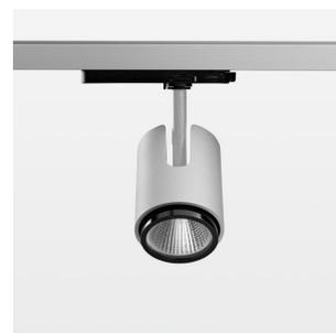
Surface-mounted luminaire with LED, rated life of the LED L80/B10 > 50000 h, chromaticity tolerance 3 SDCM (initial), reflector with circular light distribution pattern, reflector pure aluminium 99,99% in MIRO-Silver®, segmented and faceted, exchangeable reflector unit in high-shen black plastic, with glass cover, luminaire head die-cast aluminium, powder-coated, rotation angle 330°, swivel angle +/-90°, luminaire head/retention arm die-cast aluminium, stratosilver
