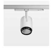
Surface-mounted luminaire with LED, rated life of the LED L80/B10 > 50000 h, chromaticity tolerance 2 SDCM (initial), , reflector with circular light distribution pattern, reflector pure aluminium 99,99% in MIRO-Silver®, segmented and faceted, exchangeable reflector unit in high-sheen black plastic, with glass cover, luminaire head die-cast aluminium, powder-coated, rotation angle 330°, swivel angle +90°/-90°, luminaire head/retention arm die-cast aluminium, special colour
