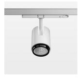
Surface-mounted luminaire with LED, rated life of the LED L80/B10 > 50000 h, chromaticity tolerance 3 SDCM (initial), , reflector with circular light distribution pattern, reflector pure aluminium 99,99% in MIRO-Silver®, segmented and faceted, exchangeable reflector unit in high-sheen black plastic, with glass cover, luminaire head die-cast aluminium, powder-coated, rotation angle 330°, swivel angle +90°/-90°, luminaire head/retention arm die-cast aluminium, special colour
