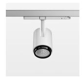
Surface-mounted luminaire with LED, rated life of the LED L80/B10 > 50000 h, chromaticity tolerance 2 SDCM (initial), , reflector with circular light distribution pattern, reflector pure aluminium 99,99% in MIRO-Silver®, segmented and faceted, exchangeable reflector unit in high-sheen black plastic, with glass cover, luminaire head die-cast aluminium, powder-coated, rotation angle 330°, swivel angle +90°/-90°, luminaire head/retention arm die-cast aluminium, special colour
