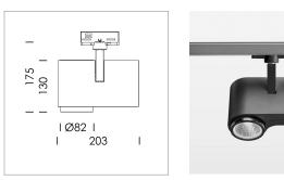
Surface-mounted luminaire with LED, rated life of the LED L80/B10 > 50000 h, colour rendering index CRI > 80, chromaticity tolerance 2 SDCM (initial), reflector with circular light distribution pattern, reflector pure aluminium 99,99% in MIRO-Silver®, segmented and faceted, exchangeable reflector unit in high-sheen black plastic, with glass cover, rotation angle 330°, swivel angle 90°, luminaire housing die-cast aluminium, powder-coated, stratoblack
