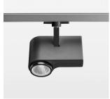
Surface-mounted luminaire with LED, rated life of the LED L80/B10 > 50000 h, colour rendering index CRI > 96, chromaticity tolerance 2 SDCM (initial), reflector with circular light distribution pattern, reflector pure aluminium 99,99% in MIRO-Silver®, segmented and faceted, exchangeable reflector unit in high-sheen black plastic, with glass cover, rotation angle 330°, swivel angle 90°, luminaire housing die-cast aluminium, powder-coated, stratoblack
